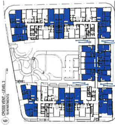
3 CROSS VENT - GROUND 18 APARTMENTS
